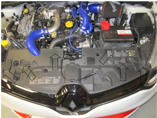
5. Disconnect the bonnet pull by pulling on the cable housing in the direction shown.
