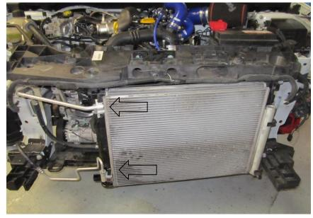
**17.** Undo the clips to the intercooler hoses.
