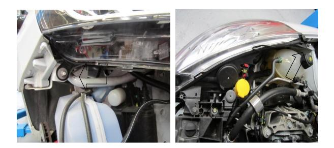
**13.** Now remove the 2 radiator clips and the 1 intercooler clip on the slam panel by turning them anti clockwise.
