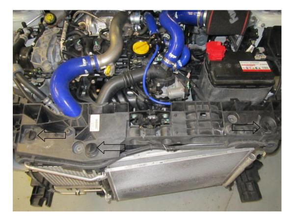
14. Using a 7mm socket remove the p clips that hold the condensor pipes in place.
