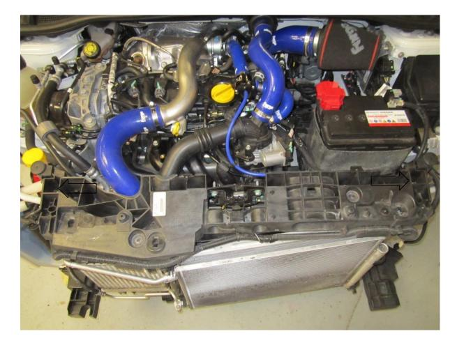
**16.** Now by pushing in the the clips on the condensorand pulling gently, remove the condensor from its locating points and slide towards the drivers side. Be careful not to damage the condensor or pipes.
