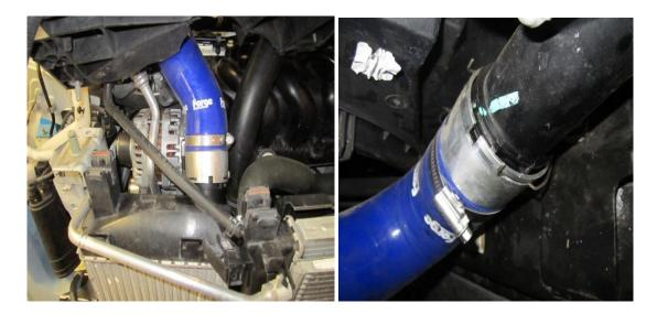
**18.** Remove the radiator overflow hose, Make sure you block this off with a bolt or your will loose all your coolant from your expansion tank.
