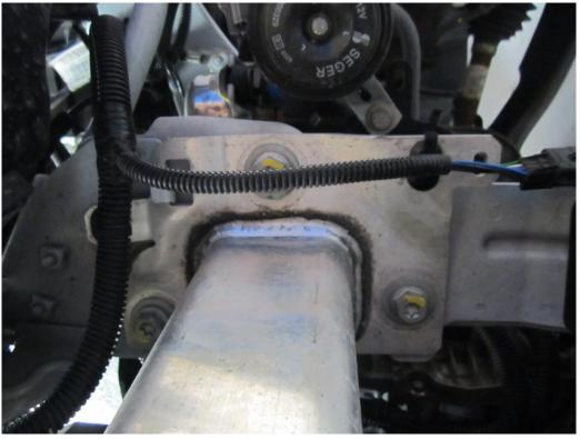
**10.** Remove the clip that holds the washer bottle neck in place.
