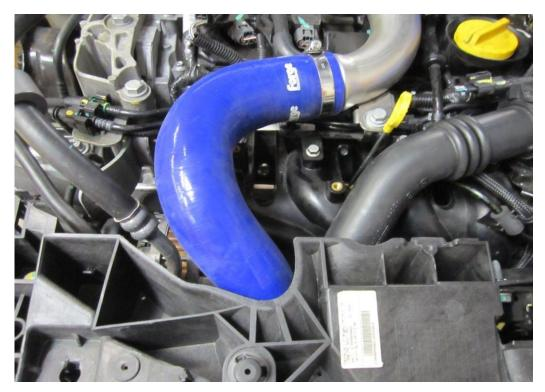
**25.** Now fit the p-clip around the hard pipe and mark your final hole to drill in the crash bar. Again use a 7mm drill bit then using your 6mm allen key and 10mm socket tighten into position .This p-clip must be fitted in order to stop the hard pipe rubbing the condensor.
